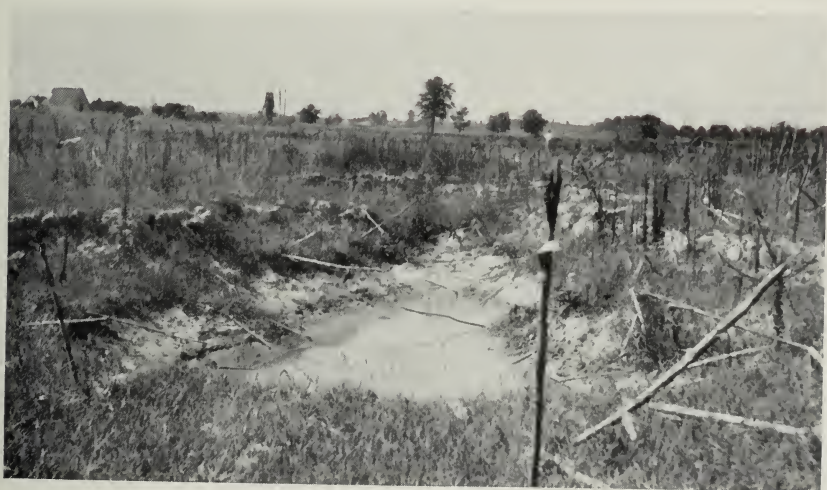
FIG. 13.—Surface breaks extending over a room in a mine near Harrisburg where the coal is 7 feet thick and 80 feet deep. The rooms are 24 feet wide and have 24-foot pillars.
